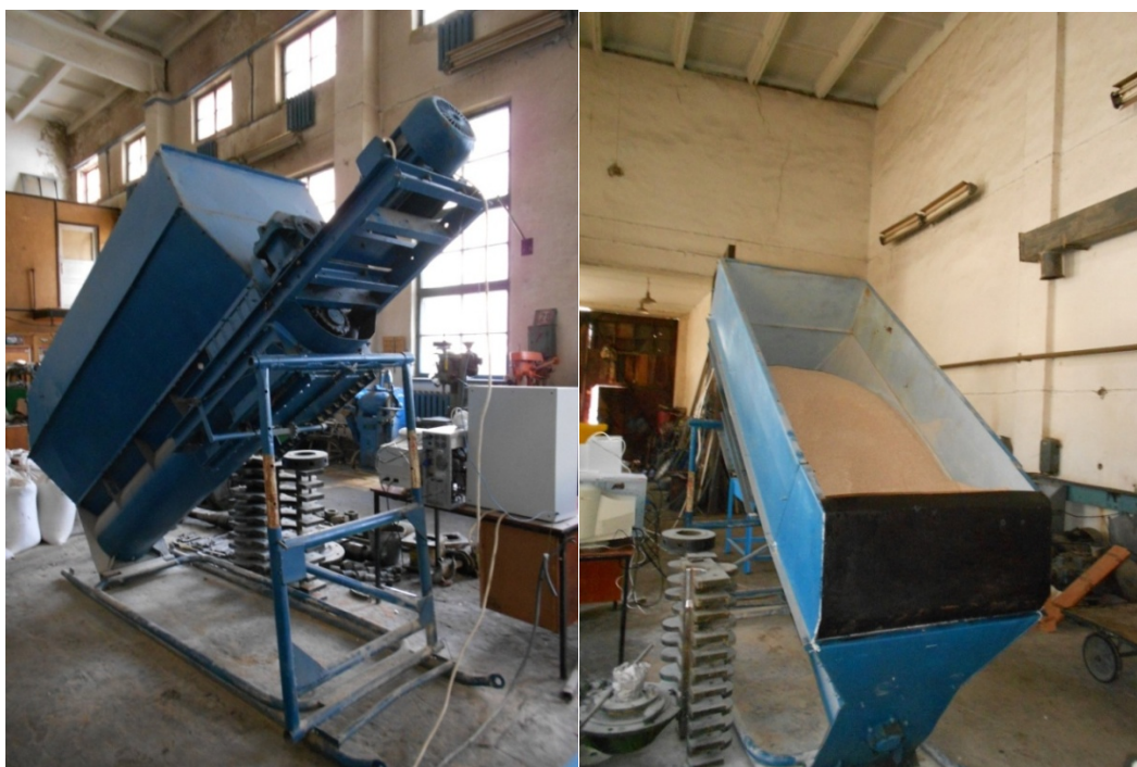
Fig. 1. General view of inclined single-screw batch mixer
