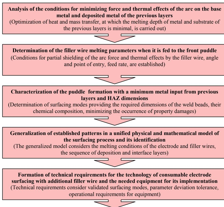
Fig. 5. Sequential algorithm for solving problems on optimizing the process of consumable electrode surfacing
