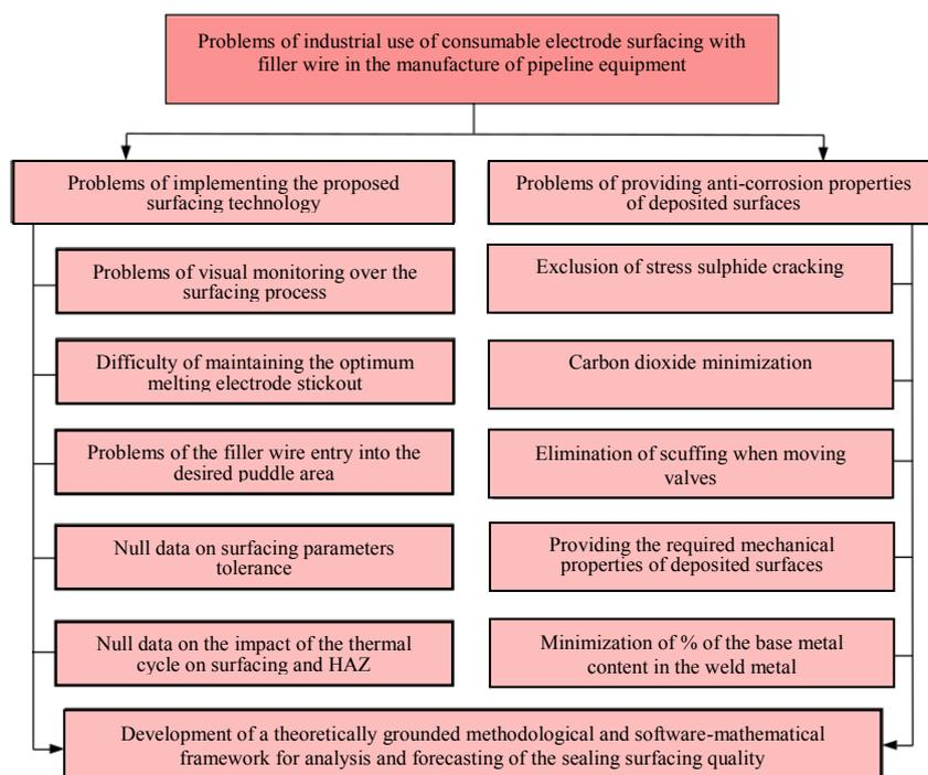
Fig. 3. Problems of industrial application of consumable electrode surfacing with an additional filler wire
