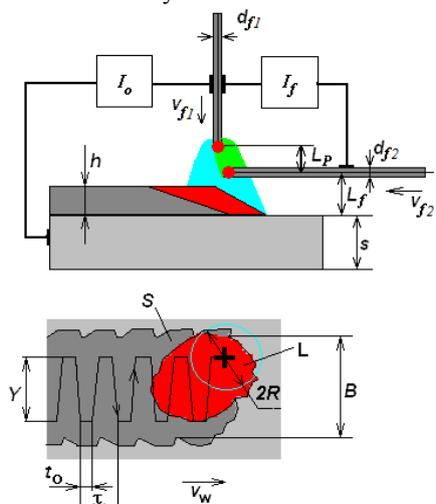
Fig. 2. Diagram of surfacing using a consumable electrode with filler wire feed and transverse oscillations of the burner:  $I_o$ ,  $I_f$  are currents of the main and additional arcs;  $R$  is the radius of the arc torch;  $s$  is the thickness of the substrate;  $d_f$ ,  $v_f$  are the diameter and wire feed speed;  $Y$ ,  $t_o$ ,  $\tau$  are parameters of transverse vibrations;  $L$ ,  $S$  are melt and overlay
